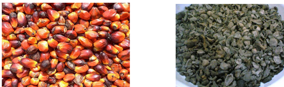
Figure 1. Palm Kernels from fresh fruit bunches (left) and Palm Kernel Shells from palm kernels (right)
